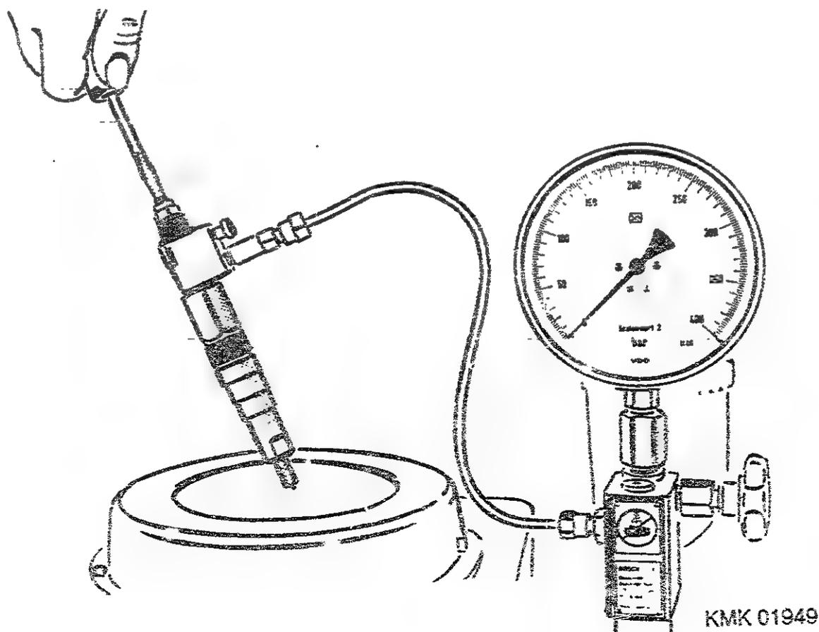
Checking hole-type nozzles and
